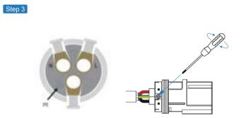
Connect AC line, Live line (L), Neutral line (N) and Ground Wire (PE) according to polarity.
