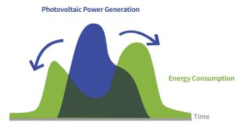
Photovoltaic energy is an unstable energy source, and the peak of power generation does not match the peak of daily electricity consumption.
